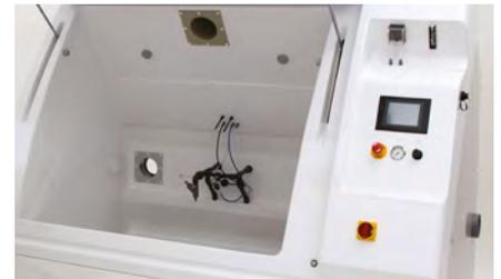
3. The Atmosfär chamber is now ready for other types of corrosion test.
