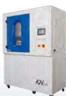
The Kesternich test is a common name for the corrosion test with sulfur dioxide (SO<sub>2</sub>) under general moisture condensation, whereby a specific volume of SO<sub>2</sub> gas, usually 0.2L, 1L or 2L is introduced into the test chamber.
