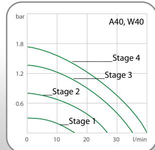
All data refers to the nominal voltage of 230 V, nominal frequency of 50 Hz and ambient temperature of +20 °C.
