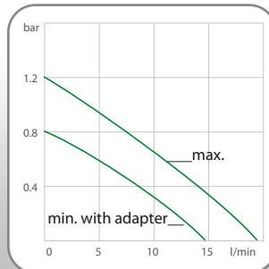
All data refers to the nominal voltage of 230 V, nominal frequency of 50 Hz (respectively 400 V, 3Ph., 50 Hz) and ambient temperature of +20 °C.
