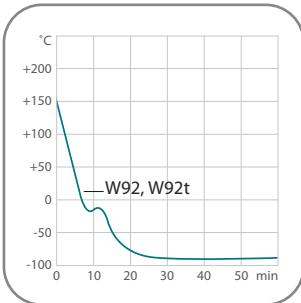
All data refers to the nominal voltage of 400 V, 3 Ph., 50 Hz and ambient temperature of +20 °C. Cooling capacity measured at max. pump stage. All pump data refers to a bath fluid with a specific density of 1 kg/dm³. Cooling capacity measured with Thermal HL (+200 °C) or Ethanol (except +200 °C)
