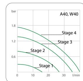
The pump capacity can be adjusted gradually or by using a pressure value (except A30). The pressure build-up is constantly monitored. Viscosity changes are compensated interactively.
